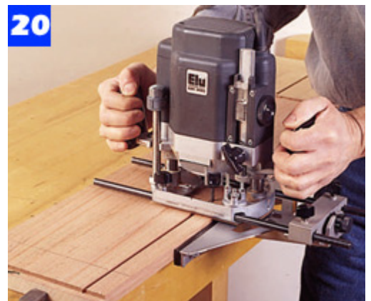
20 Install a straight bit in the router. Then, using the tool's fence, cut the drawer bottom groove in the front and sides.
