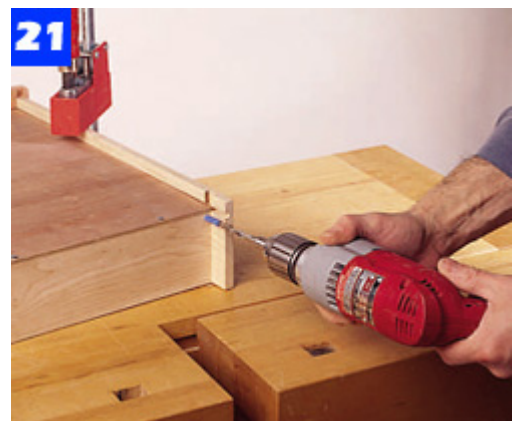
21 Use masking tape on a drill bit to mark a hole's depth, then bore the stopped holes in the back of each drawer.
