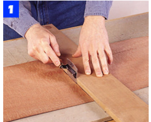
1 Place veneers on a surface into which you can cut. Slice through the stack with a veneer saw guided by a straightedge.
