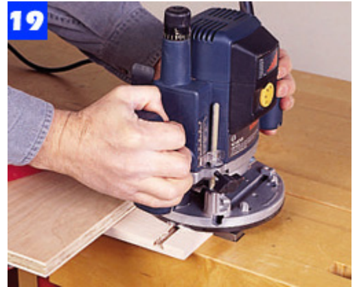
19 Cut the dovetail slots in the drawer front and sides with a router and dovetail bit. Guide the router with a straightedge.
