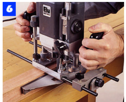
Clamp a leg securely to the bench. Using a router and straight bit, cut a stopped rabbet on the inside of the leg.
