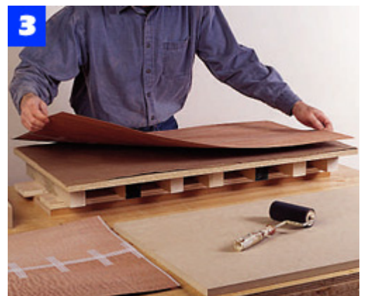
3 Place the bottom veneer facedown against a sheet of kraft paper on top of a platen, cauls and blocking.
