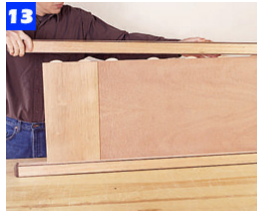
Glue and clamp together the side panels and rails. Then, test fit this assembly with the legs before gluing.
