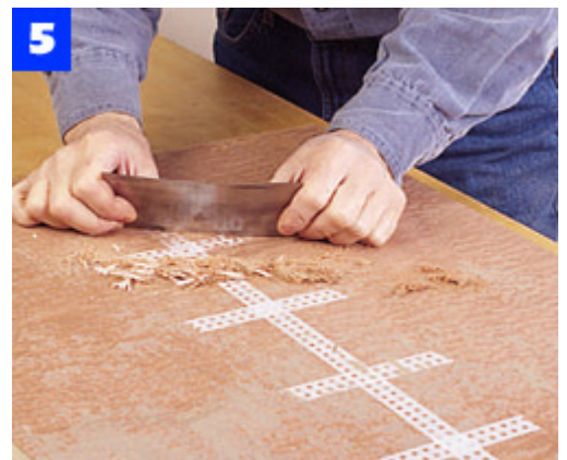
Cut the veneered panel to finished length and width, then remove the veneer tape using a sharp cabinet scraper.
