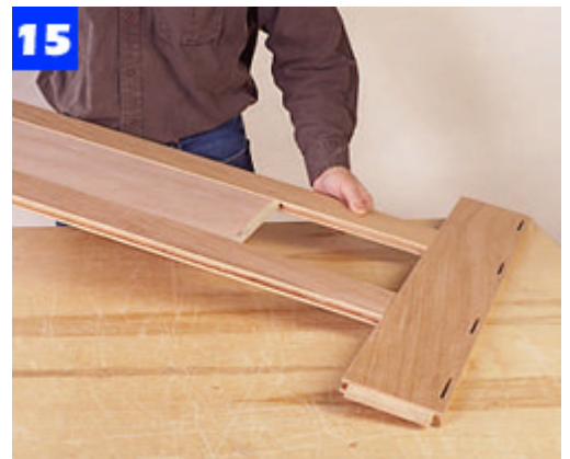
Glue and clamp together the two center stiles and one rail. Slide in the center panel before attaching the other rail.
