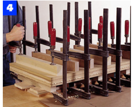
Apply clamping pressure to the veneers and core starting at the center and working outward toward the ends.
