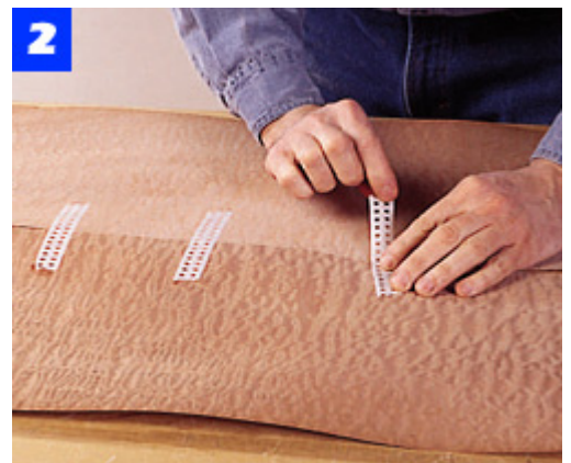
2 Make the edges of two book-matched veneers perfectly straight and smooth, then join the sheets with veneer tape.
